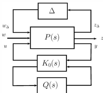
Fig. 1. Interconnection of the plant  $P(s)$  with uncertainty block  $\Delta$ , central controller  $K(s)$  and  $Q(s)$
