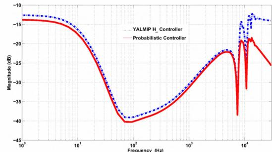
Fig. 6. Comparison between  $\mathcal{H}_\infty$  controller designed using YALMIP and proposed probabilistic controller
