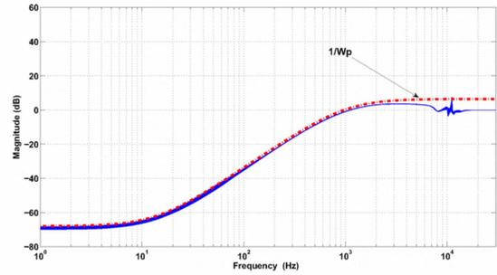
Fig. 4. Closed loop sensitivity plot with controller designed using probabilistic framework for 100 random samples of  $\Delta \in \Delta$
