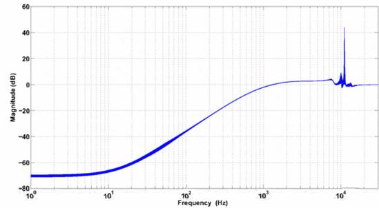
Fig. 5. Closed loop sensitivity plot with  $\mathcal{H}_\infty$  controller designed using YALMIP for 100 random samples of  $\Delta \in \Delta$
